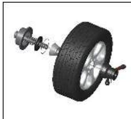
Main shaft-suitable cone(big head towards inside) —wheel—quick handle nut
