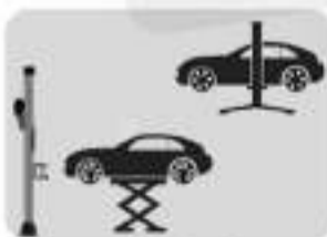
Support mini scissor lift & two post lift
